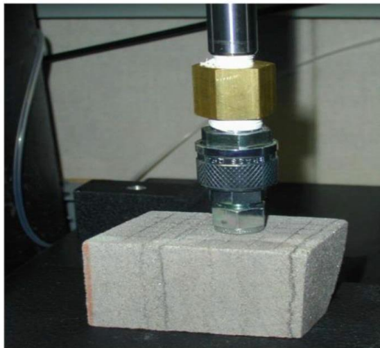
Figure 3. Probe-Permeameter During Permeability Measurements (Meyer, 2002).
